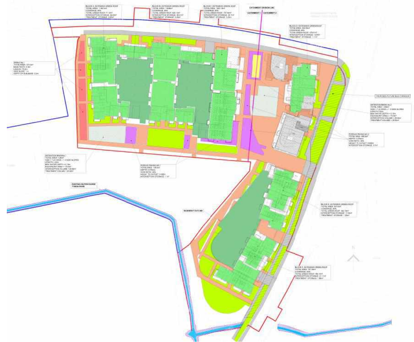
Figure 12.3 SuDS Layout (Source BMCE)
